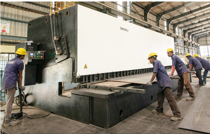
Hydraulic Shearing Machine Max.Length: 8000mm Max.Thickness: 16mm
