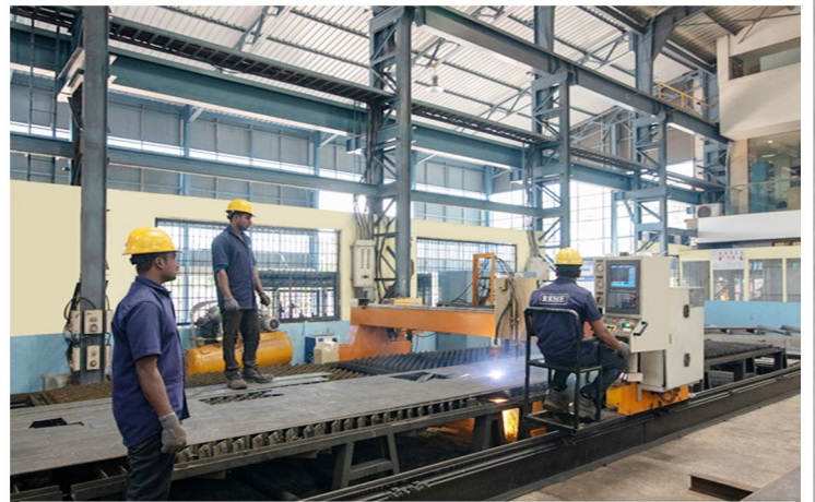
CNC Plasma & Oxy Fuel Cutting Machine Bed Size: 3000mm X 15000mm Max.Thickness: 40mm
