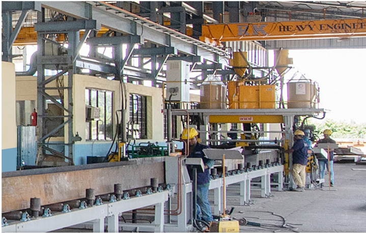
Pull Through Welding Machine (PTW) Max. Web Wide: 1500mm, Max. Web Thickness: 12mm Max.Flange Height: 450mm, Max.Flange Thickness: 20mm
