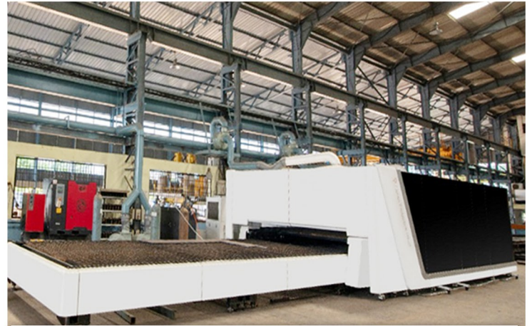
Fibre CNC Laser Cutting Machine - 4 KW BED Size: 2500mm(W) X 6100mm(L) Accuracy: 0.05mm, Max.Thickness: 20mm
